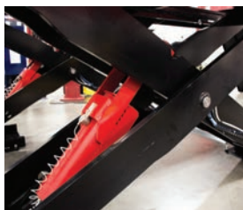
Dual hydraulic cylinders
