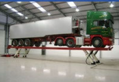
Completely vertical lifting operation
